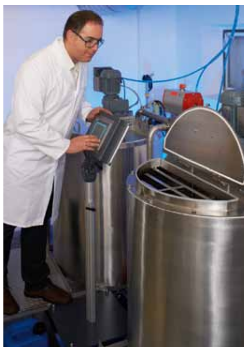
Pilot-scale reactors for synthesis of PAO-PTFE lubricants
