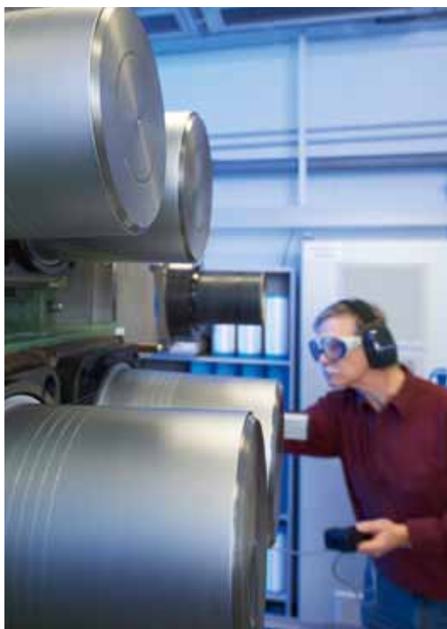
Melt-spinning plant for polymer fibres
