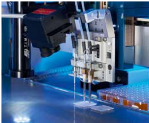
Printing of protein micro arrays in silicon cavities for multiple cell culture experiments
