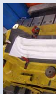
Top: Tests on industrial appliances: Deep-drawing of exterior parts for cars from sheets precoated with flexible powder coating
