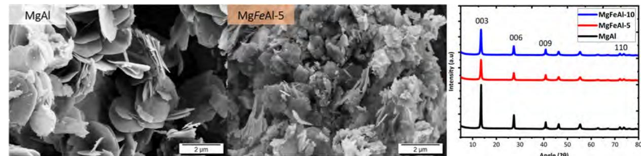
Fig. 2 SEM and XRD analysis of ternary metal (MgFeAl) LDH [6]
