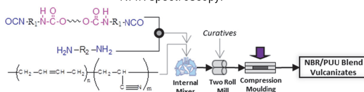
Fig. 1: Scheme of reactive blending methodology showing structure of NBR and the reactive prepolymer and diamine for the in situ PUU.
