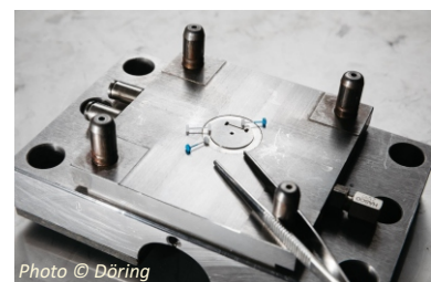
Micro tensile rod on tool insert
