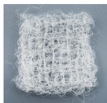
Voluminous structure by using bulk yarn
