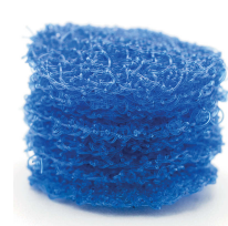
Stacked scaffold structure for long bone tissue engineering
