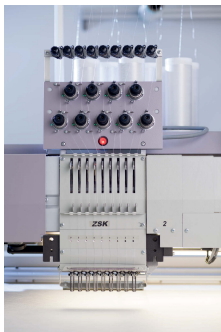
Multi-needle head for direct embroidery, different thread materials can be applied in one process
