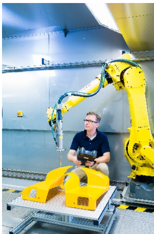
Robot controlled 3D edge- layer modification (photos: © J. Lösel)
