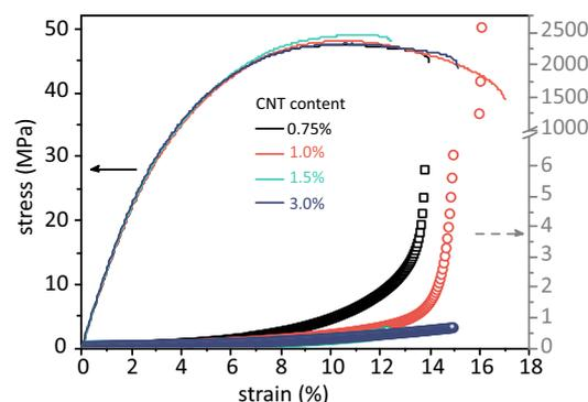
Electrical resistance change  $R_{rel}$  in stress-strain tests of PVDF composites with different CNT contents [1]
