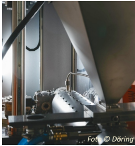
Measurement with a directly coupled plastification unit
