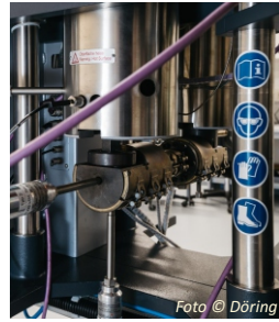
Counter-pressure chamber measurement
