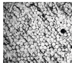
Cross sectional view showing a homogeneous fiber / matrix distribution
