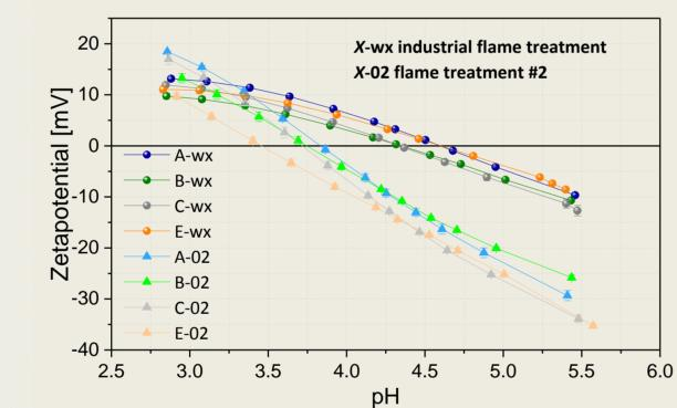
TPO surfaces treated in a paint line contained higher amounts of nitrogen resulting in a change of the acid-base properties
