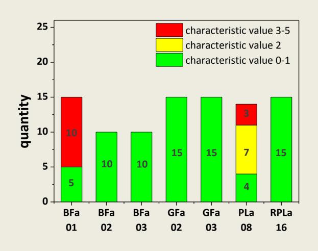
For the lowest and the highest oxygen content in the surface region of TPO, adhesion was insufficient
