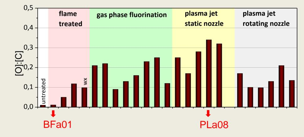
High fluctuations in the oxygen content of the outermost surface region
