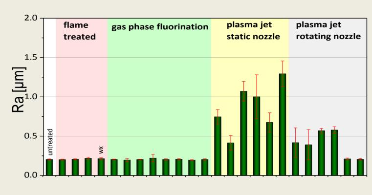
Plasma jet treatment: surface roughness and heterogeneity were dramatically increased depending on the treatment parameters
