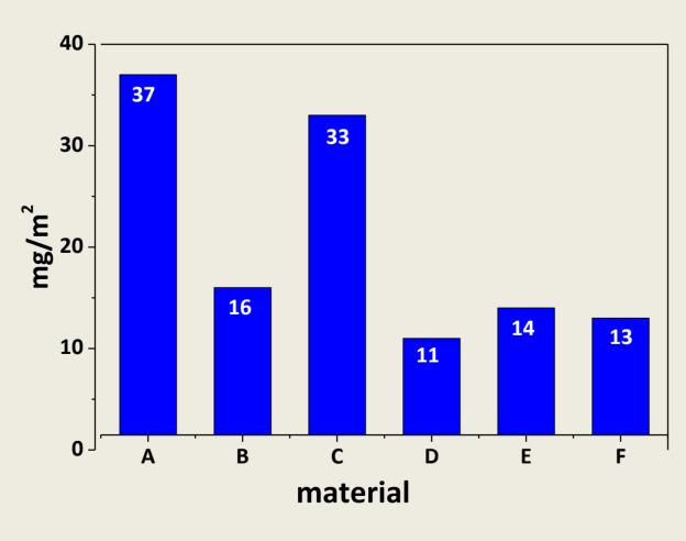
Insufficient adhesion of the paint correlates with higher amounts of soluble additives in the surface region of the different types of TPO materials
