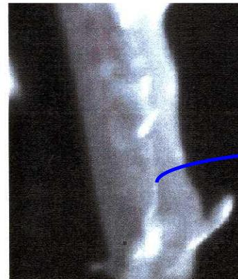
**hollow fibre of an artificial kidney cut along its length axis**
