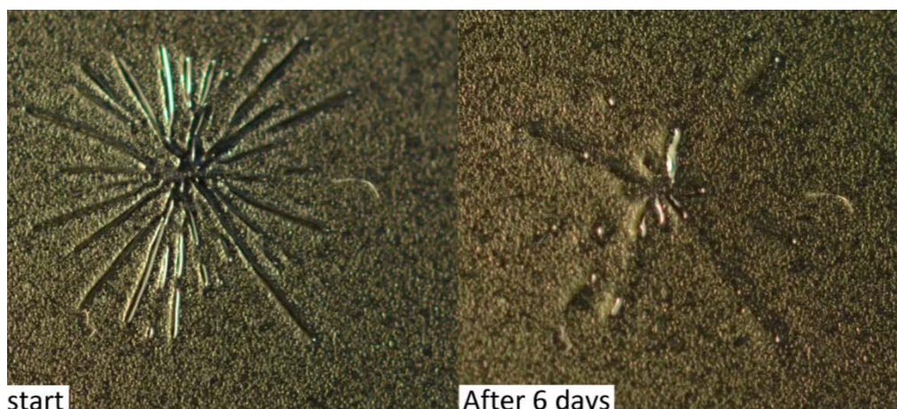
Figure 1: Self-healing of cracks in epoxy-coating (Picture: IFAM)
