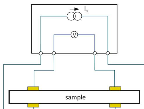
Measurement of electrical resistance
