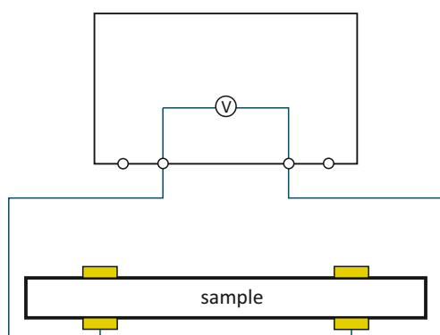
Measurement of thermoelectrical voltage
