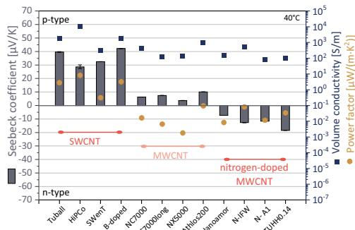
Additives to change from p-type to n-type behaviour in polymer/SWCNT composites:
