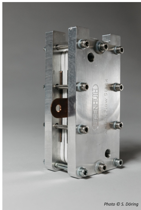
Redox flow battery stack - demonstrator of the company Eisenhuth GmbH & Co.KG
