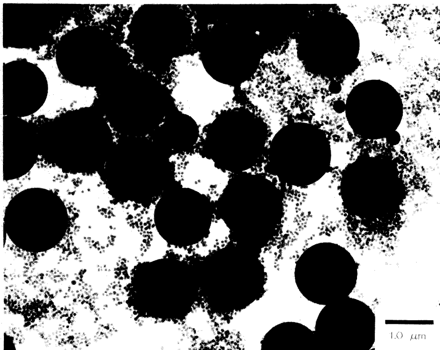
Fig. 12. Heterodisperse particle size distribution produced at 25 °C with 10 double additions of TEOS to a seed suspension prepared from 0.2 M TEOS, 1.0 M NH 3 and 5.0 M H 2 O in ethanol.
