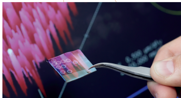
Polymeric double layer with two-dimensional gradient structured by UV light for application in self-rolling microtubes
