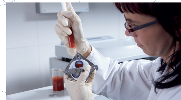
Hemocompatibility assessment: Human whole blood is filled into the screening incubation chambers
