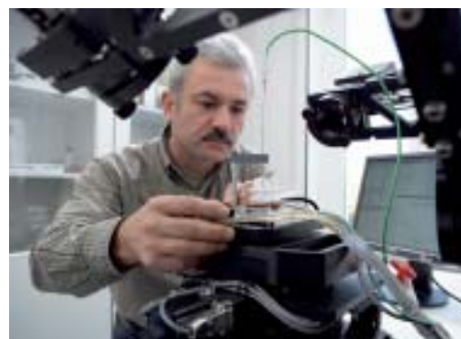
In situ spectral ellipsometry of "switchable" hydrogel layers in a temperature-controlled solid-liquid cell
