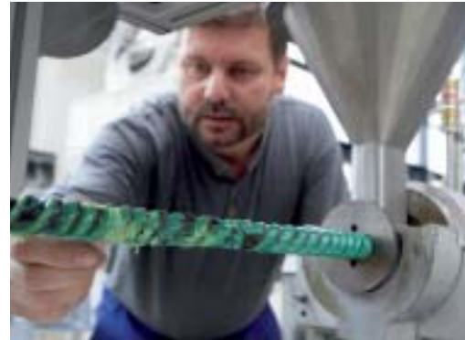
Sampling from a pair of extruder screws removed from the barrel
