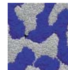
Formation of nanostructures in a binary polymer brush. The interaction between the monomers of different species causes separation processes (pattern formation) on the nanometer scale
