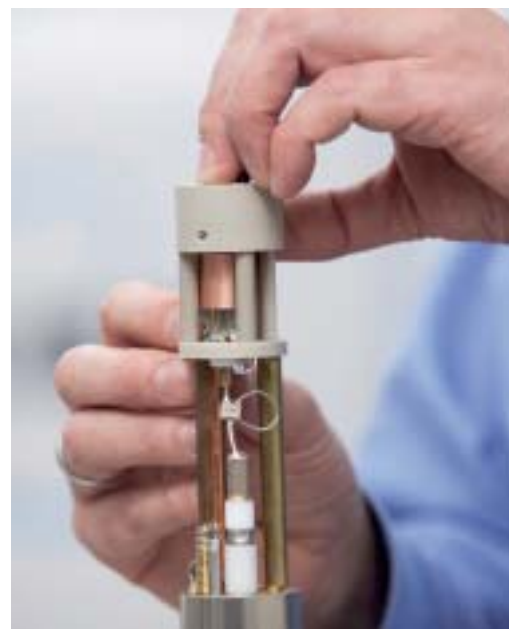
Probehead for electrophoresis NMR, developed at the IPF. Electrophoresis NMR allows to determine the charge of molecules and complexes
