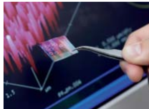
Polymeric double layer with two-dimensional gradient structured by UV light for application in self-rolling microtubes
