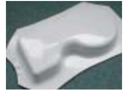
Powder-precoated aluminium sheet after deep drawing shaping test. The new uretdione powders are curable at moderate temperatures above 120 °C resulting in weather-resistant and highly flexible films
