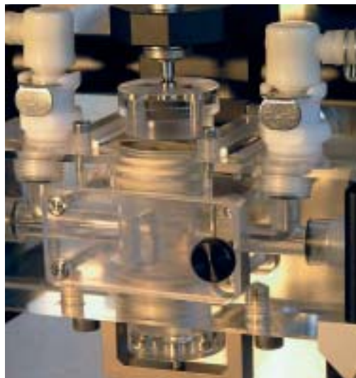
Flow cell made of PMMA with adjustable gap width for measurement of electrokinetic effects
