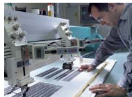
Manufacture of preforms for stress-field aligned reinforcement of components by means of a modified embroidery technology
