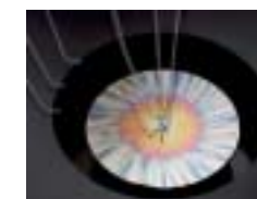
Preparation of thin polymer films from solution by means of a spin coater (cover picture)
