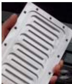
CNC machining of an aluminium plate: cut-out of a meander structure for a cooling system
