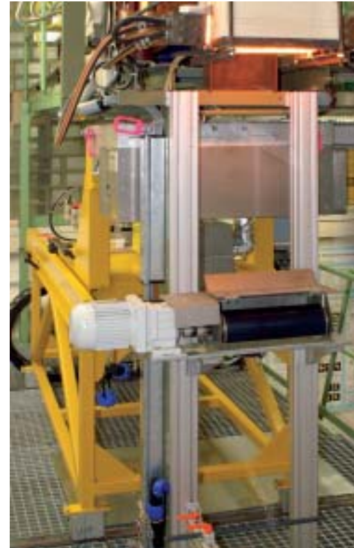
Novel equipment for online spinning of hybrid yarns (glass and polymer filaments) developed by the departments Composite Materials and Structure and Mechanics
