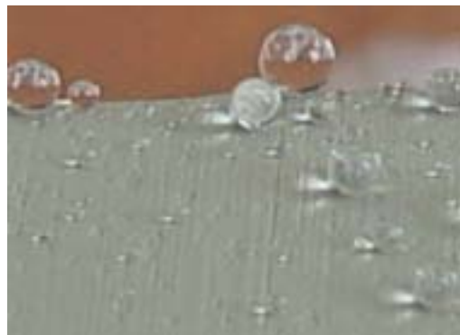
Water droplets repelled by an ultrahydrophobic aluminum substrate (Picture: K. Tittes, Nehlsen Flugzeug-galvanik GmbH)
