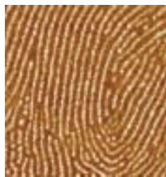
Cylindrical structure of a nanophase-separated methacrylate-based diblock copolymer
