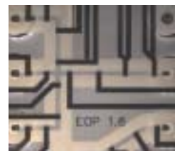
Microchannel with electrodes for electroosmotic liquid transport
