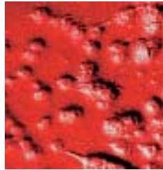
AFM height profile of a sized glass fibre (sizing compatible for polypropylene matrix, 0.4 weight-%) with single walled carbon nanotubes
