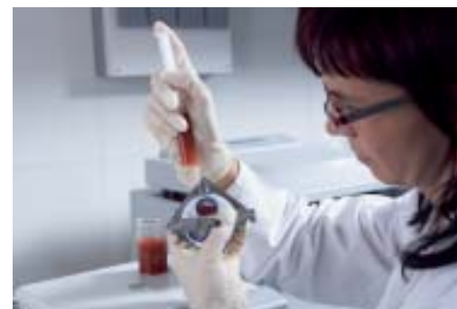
Human whole blood is filled into the screening incubation chambers for hemocompatibility assessment
