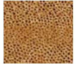
Phase morphology in a thin film (20 nm) prepared from a block copolymer based on orthogonally protected p-hydroxy styrene segments by controlled nitroxide-mediated radical polymerisation
