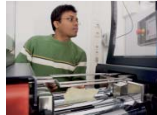
Preparation of elastomer blends using a rolling mill
