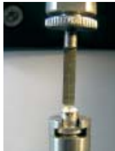
Cyclic loading in tension and compression of a glass fibre embedded in epoxy resin matrix (micro fatigue test)
