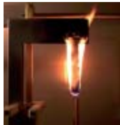
Flammability test UL 94 of a nanocomposite of polypropylene and layered silicate (filler content: 5 wt.-%)
